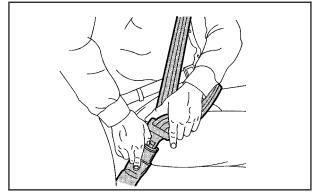
To unlatch the belt, just push the button on the buckle. For outboard seating positions, when the safety belt is not in use, slide the latch plate up the safety belt webbing. The latch plate should rest on the stitching on the safety belt, near the guide loop on the side wall.
